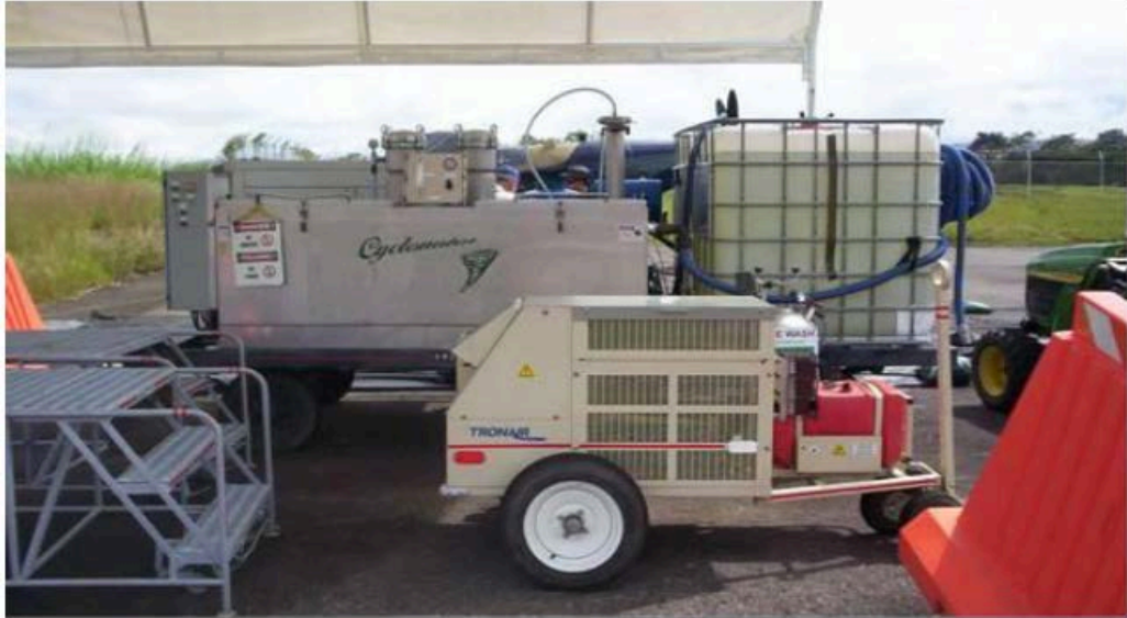
Image 18: Treatment Plant for Industrial Liquid Waste from Washing the Aircraft
