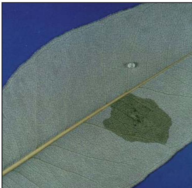
Photo 6. Comparison between a drop of water without (top) and with (bottom) the addition of a surfactant. Addition of the surfactant greatly increased the spreading ability of the water droplet.
